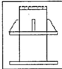
Consists of 4 units in a set, typically 2,210 mm (87.0 in) in height, cast into the concrete with approximately 305 mm (12.0 in) protrusion above the concrete surface. The starter legs are normally set in by using the first tower section as template.
