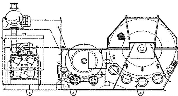
Winches consist of parallel grooved drums for hoist and luff motion. Each drum is driven by fixed or variable displacement hydraulic motors, which through oil immersed disc brake and multiple planetary gearboxes and pinion, drive the external drum gear.
