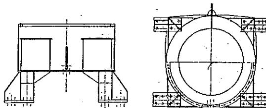
The slew mount is a rigid welded structure which is bolted to the crane tower and to which the slew bearing is fastened. The slew bearing has an integral gear to provide a drive via a hydraulic motor and gearbox situated on the machinery deck.
