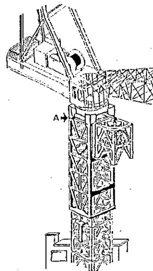
Internal Ladder Climbing Frame with 32 m (105 ft) ladder and 3 sets of collars
