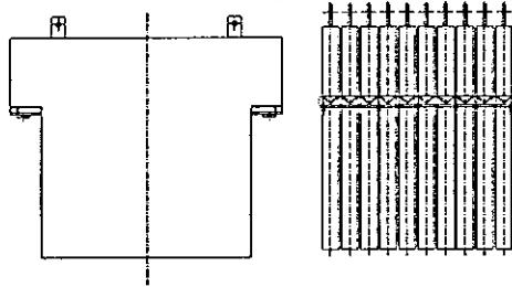
The counterweights of 65,000 kg (143,300 lb) consist of heavy steel plate or concrete sections, which are supported on the rear of the machinery deck.
