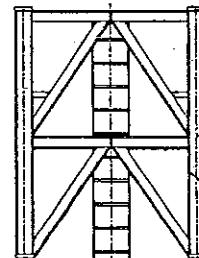
Tower sections are of welded construction and are braced for maximum torsional bending strength. Connection is made by high tensile steel bolts at each corner, developing the full strength of each corner. The tower sections have included a platform and ladders to provide access to machinery deck.
