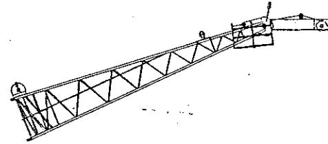
This 3.1m (10.2 ft) fly jib section is pinned to the end of the boom top section at an offset of 30°.
