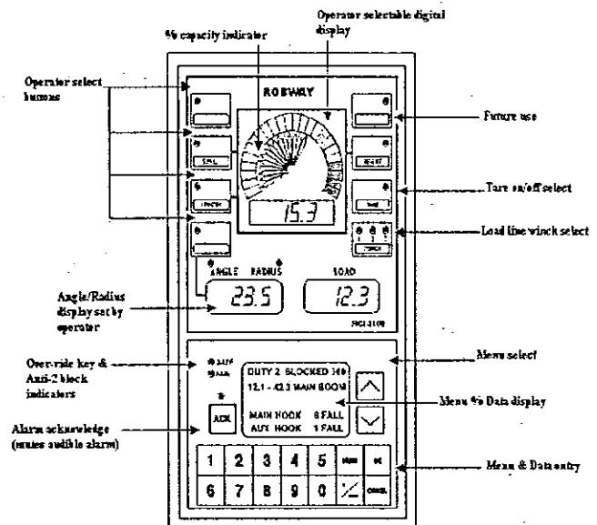
The RCI-3100 automatic Rated Capacity Indicator (RCI) is designed to assist the operator in the course of normal crane operation and consists of boom angle, length and slew.
