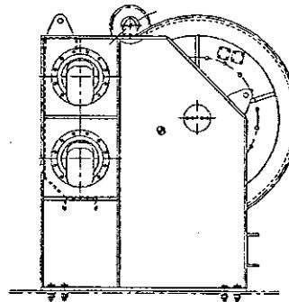
12 t (26,456 lb) fly winch using 32 mm (1 1/4 in) rope lifting 12,000 kg (26,456 lb) on a single fall hook.
