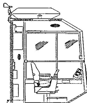
The cabin can be mounted on either side of the machinery deck.
